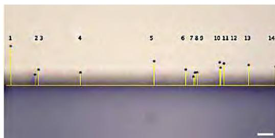
*Figure 4: Accuracy of bead placement was quantified by measuring the distance between dispensed beads and the intended patterning target. Scale bar is 100  $\mu\text{m}$ . To acquire this image, a human hair was taped to the bottom of the sample container and used as a linear target.*
