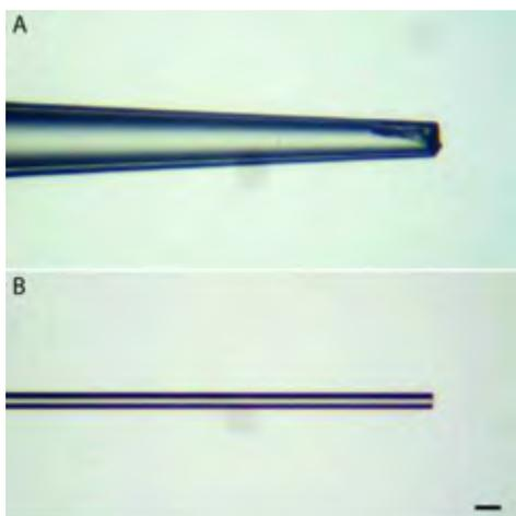
*Figure 2: Micropipettes produced by standard protocol (A) and with custom weights (B). Scale bar is 50  $\mu\text{m}$ .*
