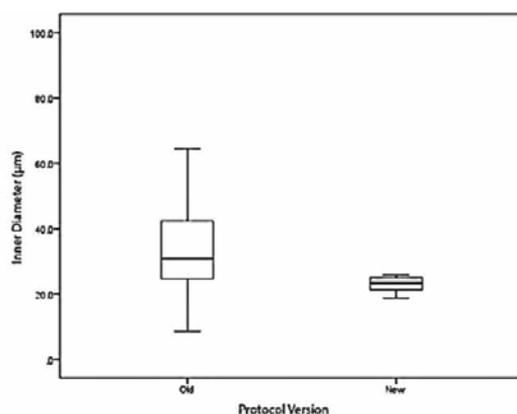
*Figure 3: Box plot comparing micropipette diameters resulting from pulls performed using standard and custom equipment.*
