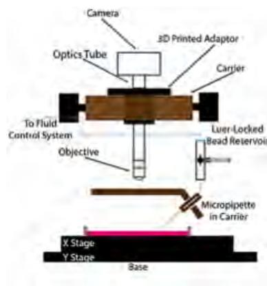
**Figure 1:** Schematic of the microbead-dispensing instrument. An upright microscope is used to visualize the bead-filled glass micropipette, which is driven by a syringe pump. A motorized XY stage is used to manipulate the sample container, facilitating reproducible bead patterning.
